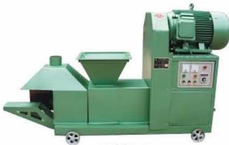
ZBJ-I capacity: 150-200kg/h power: 7.5-11kw
